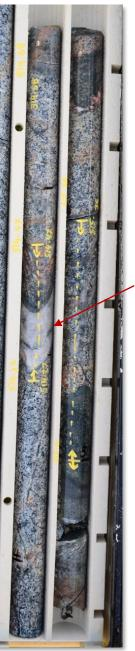
Diamond drilling intercepted two structures: - E07 Hanging wall (-514.27m) - New E07 Footwall (-589.5m)
