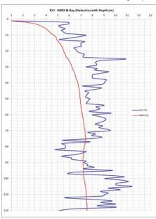
Figure 2. An example of virtual bore dielectrics from a project looking at aquifers
